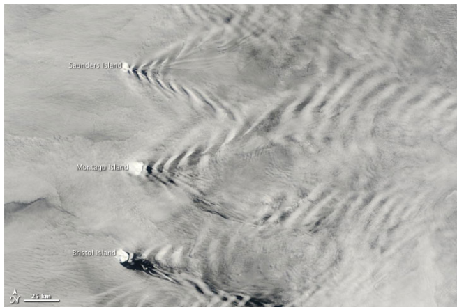
Figure: Satellite imagery showing three-dimensional trapped lee waves induced by the Sandwich Islands in southern Atlantic Ocean on November 23, 2009. The wave pattern is similar to that of the ship waves. (credit: NASA)
