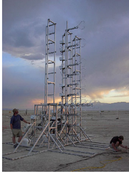
Figure 2. Photograph of the field study setup at the SLTEST facility on the salt flats in Western Utah. The setup consists of 16 sonic anemometers positioned along vertical and horizontal arrays, crossing at 1.9 m above the desert floor.
