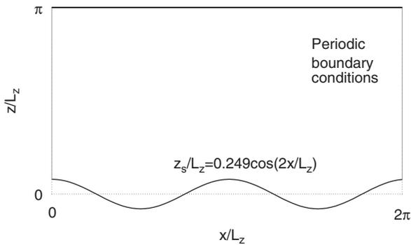
Fig. 1. Schematic of computational domain over the sinusoidal hill.
