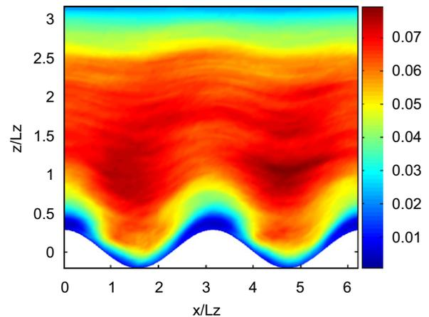
Fig. 6. Smagorinsky coefficient ( $C_s^2$ ) obtained with the scale-dependent Lagrangian dynamic model. Results are averaged over time and spanwise direction.
