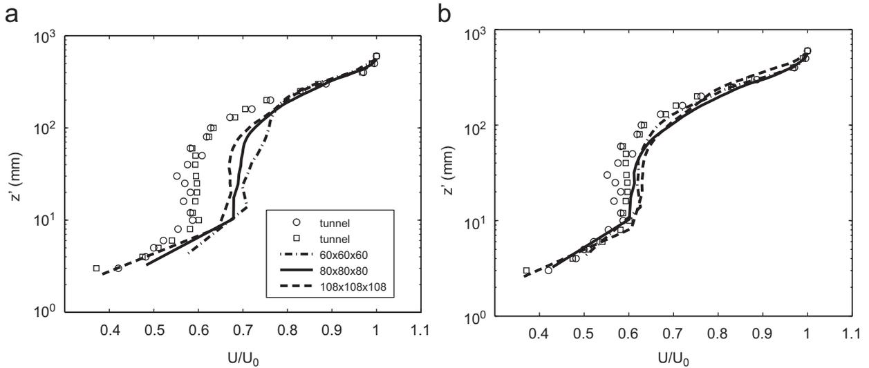
Fig. 4. Effect of grid resolution on the simulated non-dimensional velocity profile over the wave crest obtained with the Lagrangian dynamic model (a) and the scale-dependent Lagrangian dynamic model (b). The wind tunnel data of Gong et al. (1996) (symbols) are also shown.
