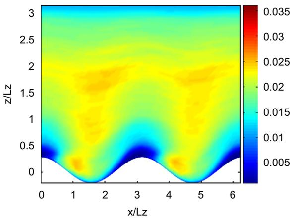
Fig. 5. Smagorinsky coefficient ( $C_s^2$ ) obtained with the Lagrangian dynamic model. Results are averaged over time and spanwise direction.
