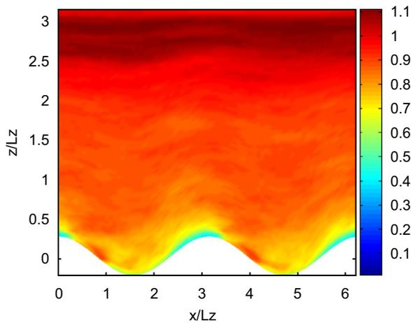
Fig. 7. Scale dependence parameter ( $\beta$ ) obtained with the scale-dependent Lagrangian dynamic model. Results are averaged over time and spanwise direction.
