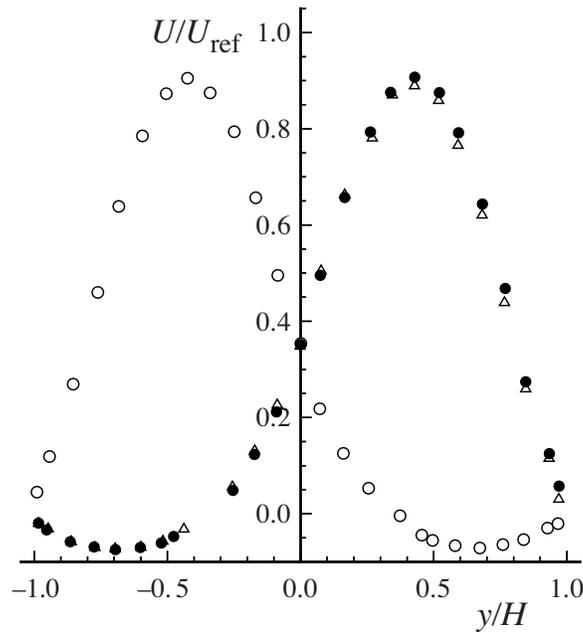
Fig. 3.26. Velocity profiles measured by Durst *et al.* (1974) in the steady laminar flow downstream of a symmetric expansion in a rectangular duct. The geometry and boundary conditions are symmetric about the plane  $y = 0$ . Symbols:  $\circ$ , stable state 1;  $\triangle$ , stable state 2;  $\bullet$ , reflection of profile 1 about the  $y$  axis.
