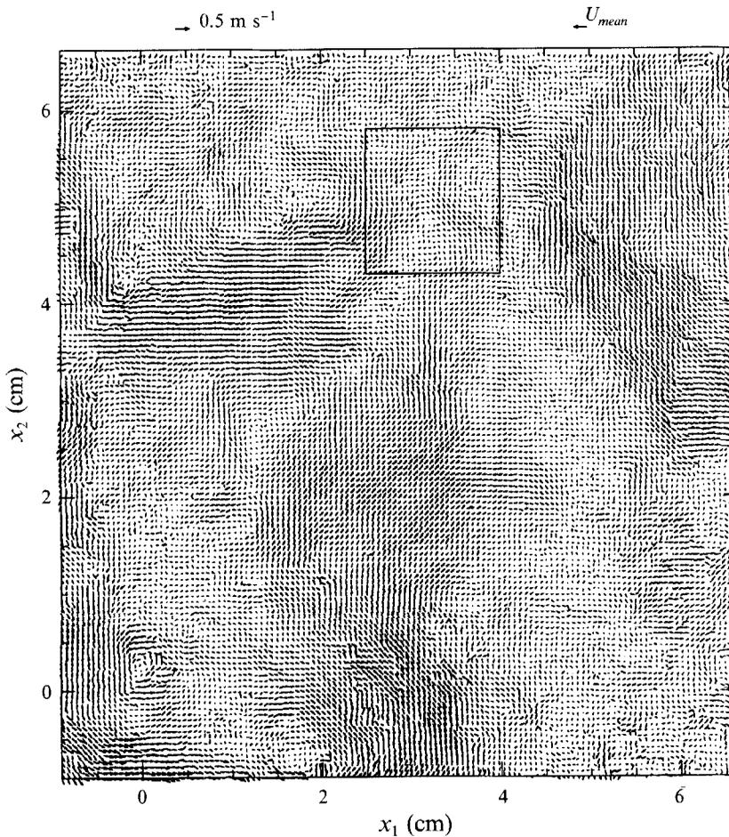
FIGURE 2. Instantaneous velocity vectors projected onto an axial plane in the far field of a turbulent round jet. There are  $128 \times 128$  vectors. The mean velocity of the image (shown on the top right) is from right to left, and has been subtracted from each vector. The velocity scale is indicated on the top left.
