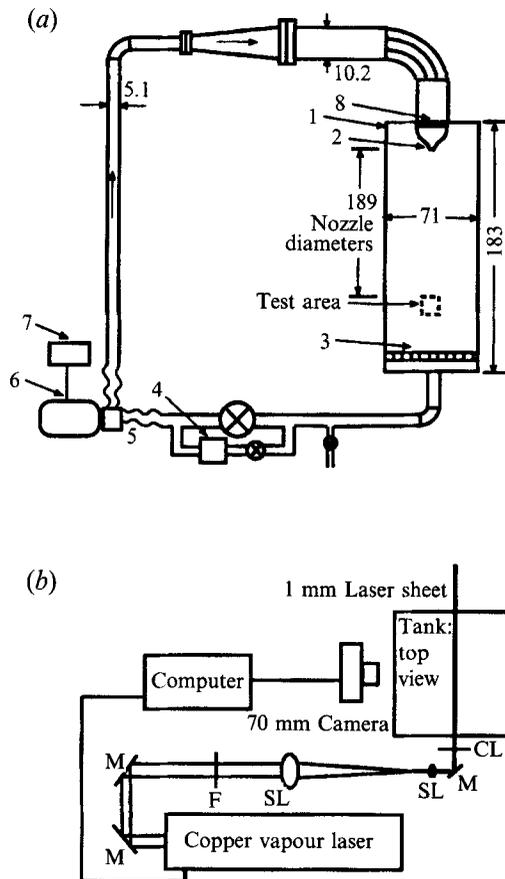
FIGURE 1. Schematic of the experimental set-up. The facility is shown in (a): 1, tank; 2, nozzle ( $D = 0.635$  cm); 3, honeycomb; 4, filter; 5, flexible hose; 6, pump; 7, speed control; 8, honeycomb & screen. All dimensions are in cm. The optical instrumentation is shown in (b): M, mirror; SL, spherical lens; CL, cylindrical lens; F, filter.
