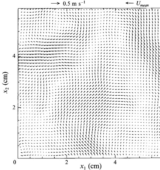
FIGURE 5. Vector map of the filtered velocity  $\tilde{u}_i$ . A top-hat filter was applied to the image shown in figure 2, with a width  $\Delta = 8\delta \sim 48\eta$ , where  $\delta$  is the original grid size (0.55 mm) and  $\eta$  is the Kolmogorov scale. To avoid crowding, the figure shows every second vector only. The mean velocity and the fundamental velocity unit is shown on the top.
