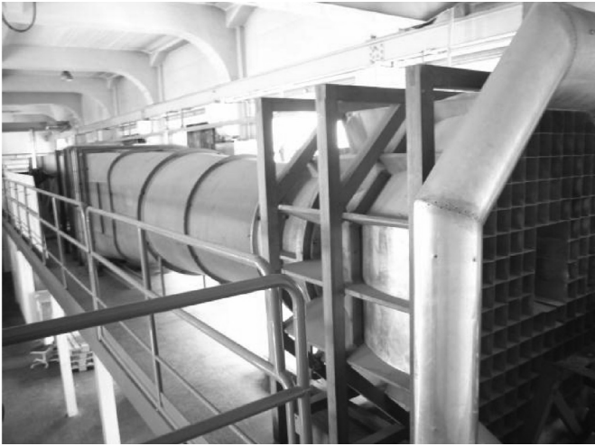
Figure 2.4 Picture of the Rauhgigkeitskanal at the Max Planck Institute for Dynamics and Self-Organization. It was built in 1935 and reconstituted by Helmut Eckelmann and James Wallace in the 1970s.
