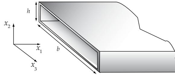
Fig. 3.25. A sketch of a turbulent-channel-flow apparatus.
