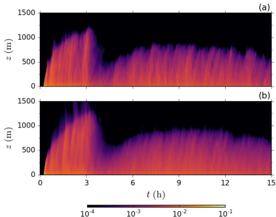
**Figure:** TKE from DNS of a low-level jet. (a) and (b) have different slope angles.
