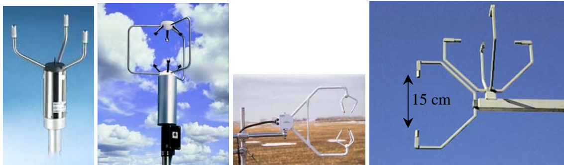
Fig. 1: Various sonic anemometer configurations: (a) 2D sonic anemometer with vertical mounting base, (b) 3D SAT with vertical mounting base, (c) 3D SAT with horizontal mounting non-orthogonal pulse paths, (d) 3D SAT with horizontal mounting and orthogonal pulse paths. Photographs are courtesy of (a) Vaisala, Inc. (b) RM Young Company, (c) Campbell Scientific, Inc. and (d) Applied technologies, Inc.
